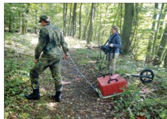
Fig. 3: Ground-penetrating radar measurement with a 200-MHz antenna (red box) near Breitenbenden (Eifel hills). The underground Roman aqueduct (which is now dry) was looked for and found in this forest area
