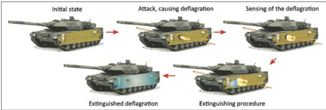
Fig. 3: Functional principle of a fire suppression system
