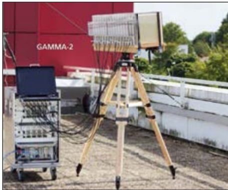
Fig. 2: Experimental 16-channel passive radar system that uses mobile phone base stations (GSM broadcast signal) for drone illumination
