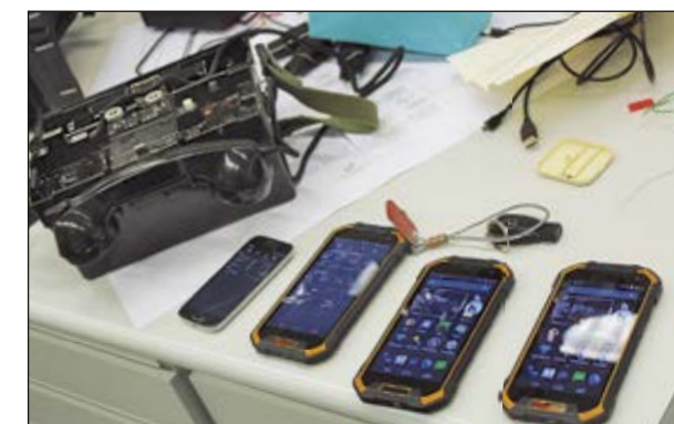
Fig. 3: Successful integration of legacy communication equipment into the modern LTE over Satellite network. VoIP connectivity was reliably established between a field telephone (FFOBZB), manufactured in 1956, and the modern LTE user equipment running on the Android operating system
