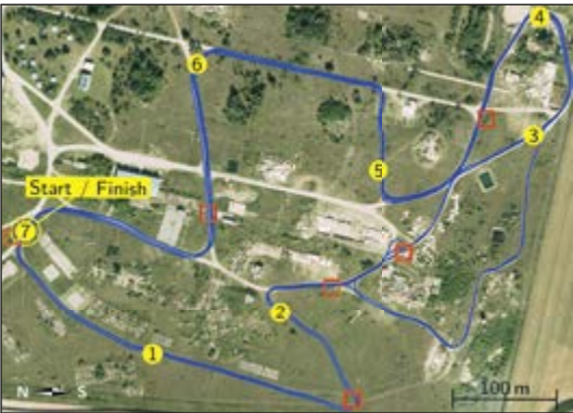
Fig. 1: Convoy scenario of M-ELROB 2016: aerial image of the competition area showing the path driven (blue), waypoints in a pre-given order (yellow) and mapped warning signs (orange)
