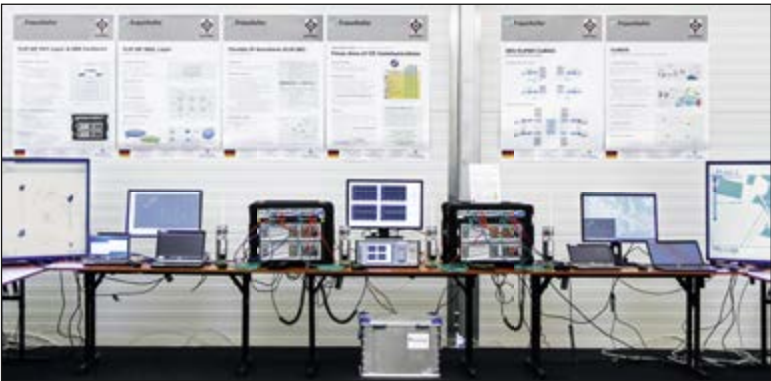
Fig. 2: Diagram of the CWIX 2016 test set-up comprising the two test systems (black cubes) and the channel emulator (centre); (Source: Joint Force Training Centre (JFTC) Bydgoszcz)
