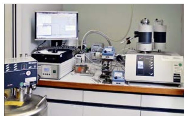
Fig. 1: Simultaneous thermal analysis (STA) apparatus for performing TG-DSC measurements
