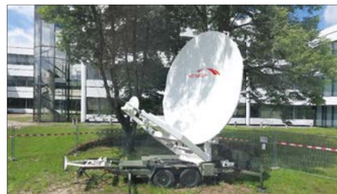
Fig. 2: Hub station (4.6 m) as part of the SatCERTBw reference facility in operation during the demonstration of LTE over Satellite
