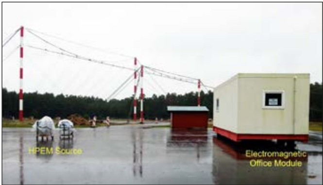
Fig. 1: EM office module exposed to an HPEM interference source
