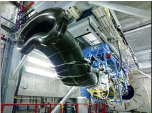
Fig. 2: The MEIRD research duct installed upstream of a Larzac 04 turbofan engine in the engine test facility at the Institute of Jet Propulsion
