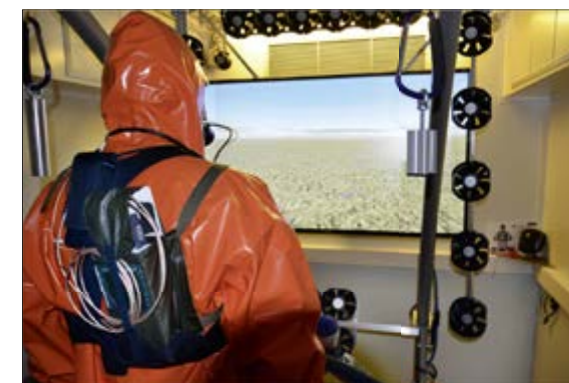
Fig. 4: Volunteer in thermally insulating protective clothing in a climatic chamber
