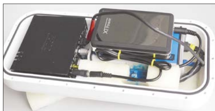
Fig. 2: Pressure-resistant housing with electronics: potentiostat, mini-PC, pump driver, power supply
