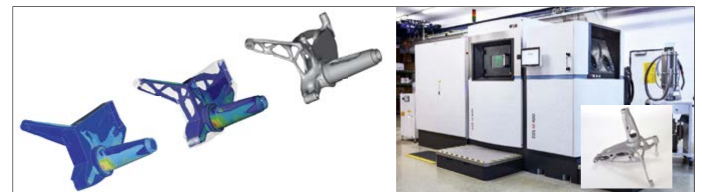
Fig. 2: Numerical design optimisation for a wheel carrier, and 3D printing of the final design using the direct metal laser sintering system at Fraunhofer EMI, for testing and experimentation
