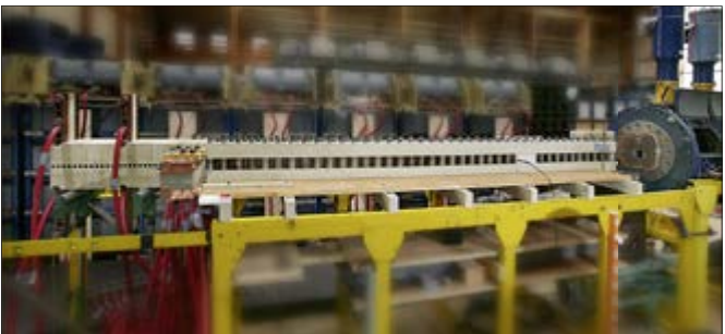
Fig. 4: 25 mm calibre railgun capable of firing bursts
