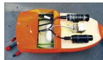
Fig. 3: Sensor system integrated inside the payload compartment of the SeaCat, of Atlas Elektronik
