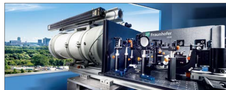
Fig. 3: Transportable measuring setup for characterising and correcting atmospheric turbulence
