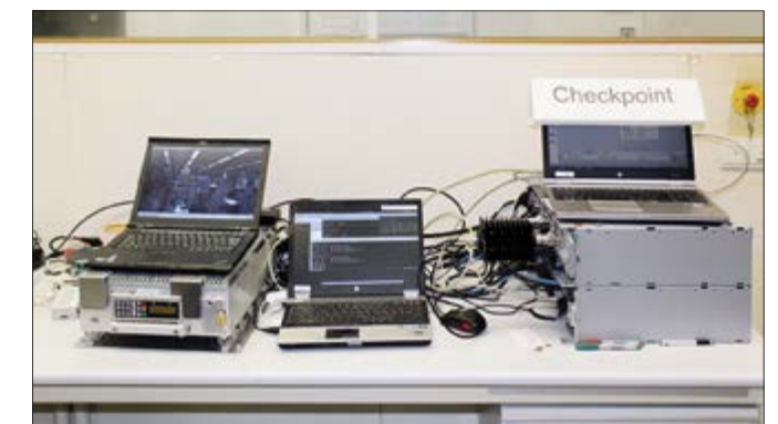
Fig. 4: Integration of a Sina Box into the network during the demonstration at Universität der Bundeswehr München. Left: Sina Box with SECRET classified tunnel and live video transmission via satellite; centre: LTE core network components installed in a commercial laptop; right: LTE base station (eNodeB)
