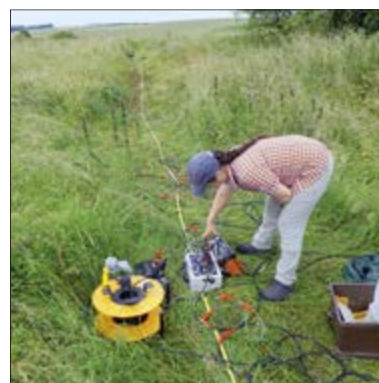
Fig. 2: Goelectricity measurement in the La Boisselle measuring area, France. The exact location of the mining galleries was unknown in this case
