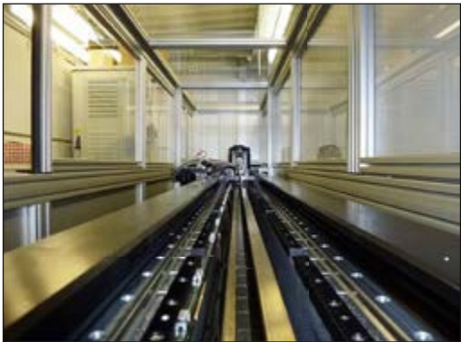
Fig. 2: Linear stage in the receiving station of the atmospheric propagation test range
