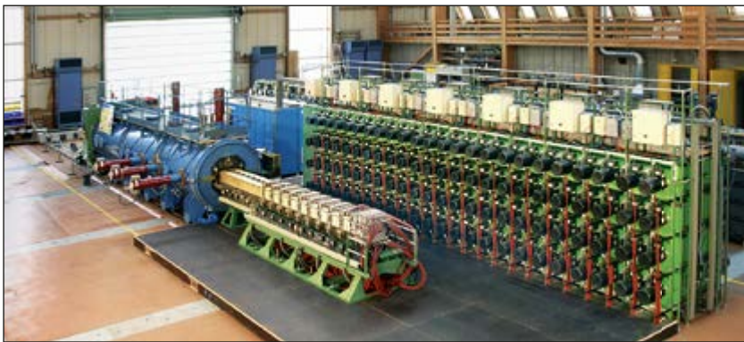
Fig. 1: 40 mm calibre ISL railgun with a 10 MJ power supply
