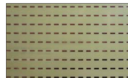
Fig. 4: A frequency- and polarisation-selective meta-sheet realised as a periodic array of copper strips printed on top of FR4 substrate
